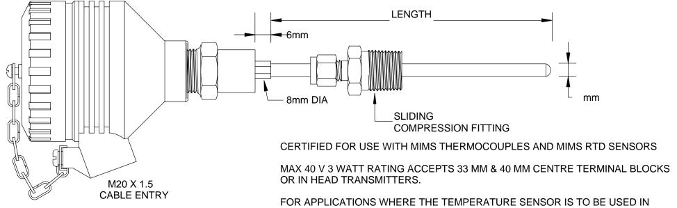
FOR APPLICATIONS WHERE THE TEMPERATURE SENSOR IS TO BE USED IN T5 TO T1 TEMPERATURES A 50 MM LAGGING EXTENSION SHALL BE FITTED TO ENSURE THE ENCLOSURE REMAINS BELOW T6 TEMPERATURE RATING.
